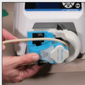
2. Place tubing over rollers and through retainers.
